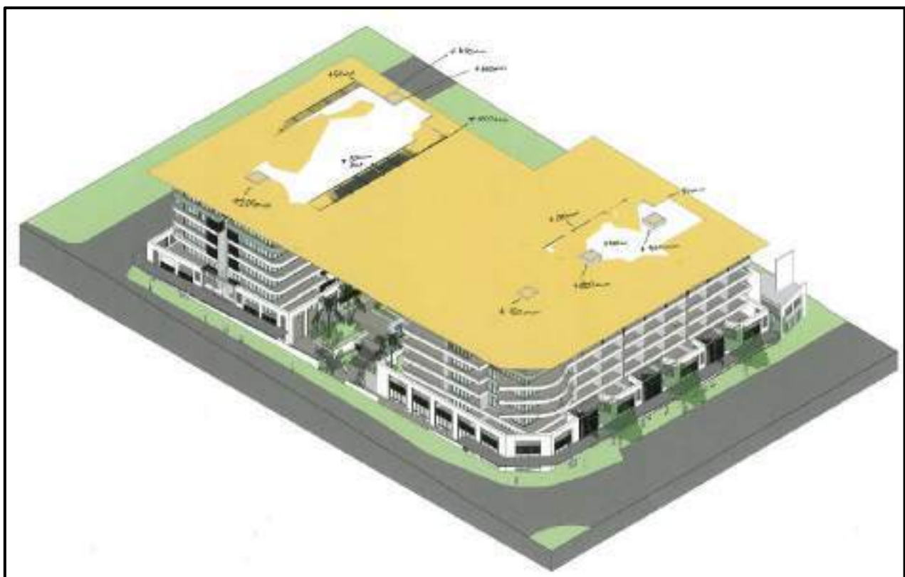
Figure 7: Height of building encroachments.
